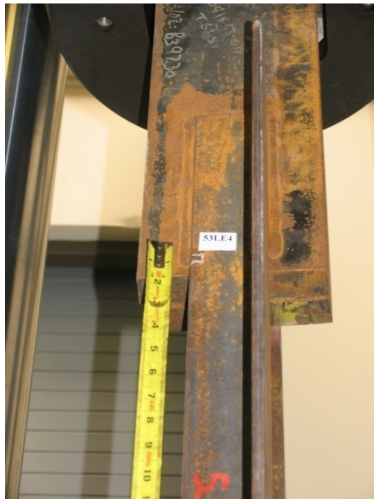
Figure 51. 53LE Angle Failure Close-Up
