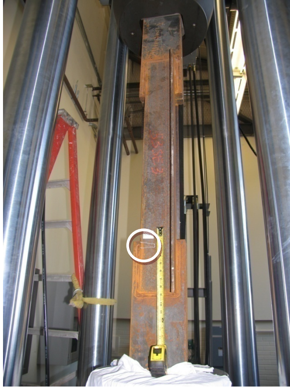
Figure 45. 53SE Angle Failure
