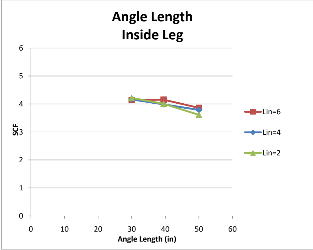
Figure 103. Angle Length and Inside Leg Length vs. Stress Concentration Factor
