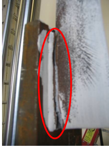
Figure 32. Typical Static Failure of Weld
