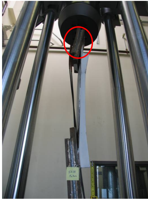
Figure 30. Failed Specimen (failure is circled)
