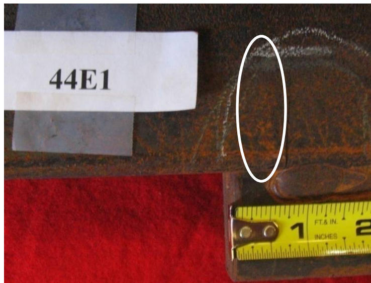
Figure 23. Close-Up of Cracked Specimen
