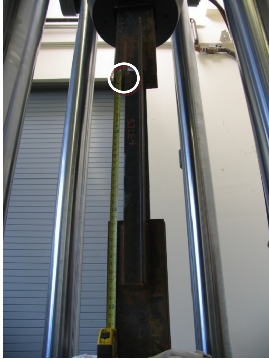
Figure 50. 53LE Angle Failure
