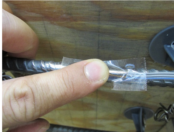
Figure 8 – Pressure applied to strain gage and adhesive
