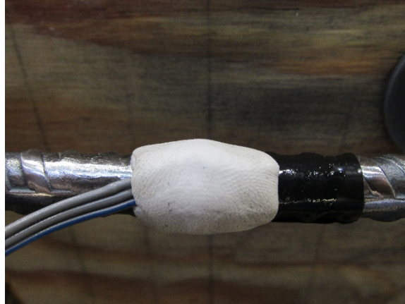
Figure 14 – Lead wire encapsulated in SB tape
