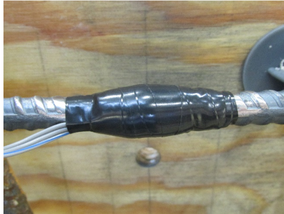
Figure 16 – Strain gage and bar covered with electrical tape
