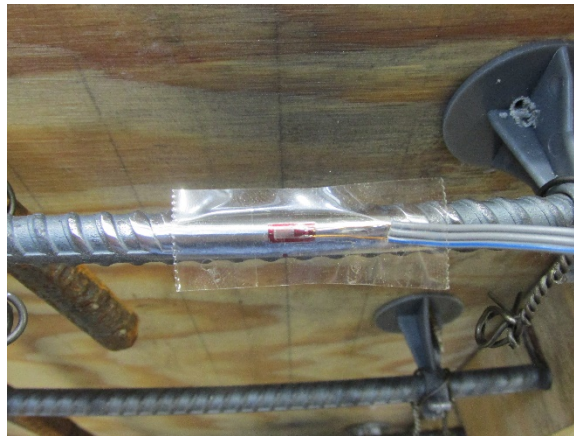
Figure 5 – Strain gage held in position with tape
