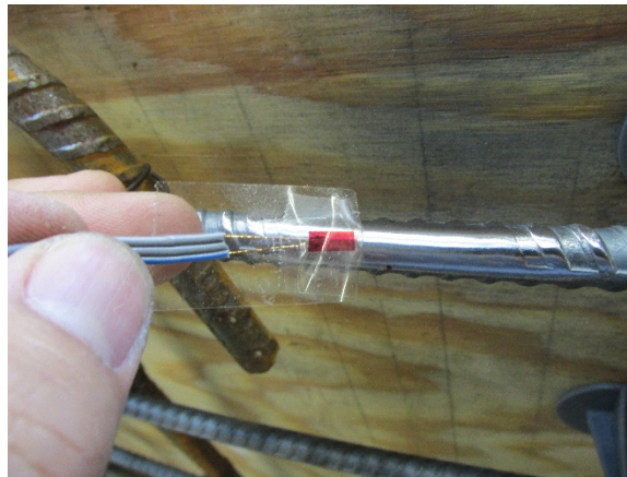
Figure 6 – Strain gage and tape peeled back for gluing
