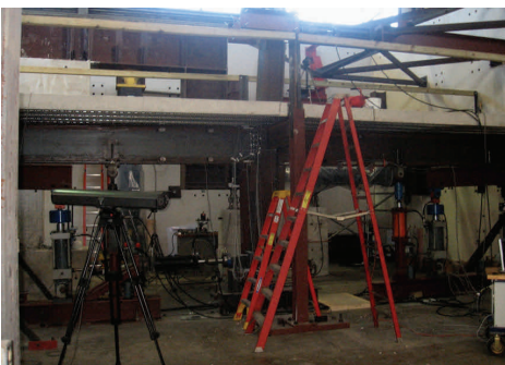
Test setup at 9% inter-story drift
