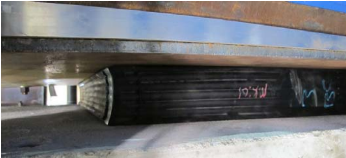
Bearing tested under axial load and rotation
