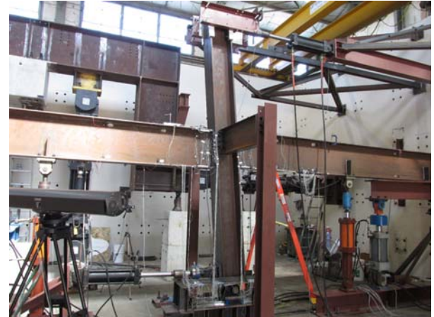
Test setup at 9% inter-story drift
