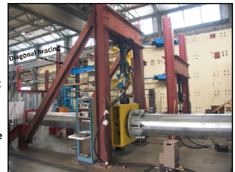
Portal loading frame used in previous fatigue studies in HMIPs at Ferguson Lab
