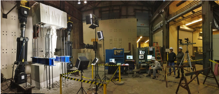
Test setup and CS100 specimen at the end of the test.
