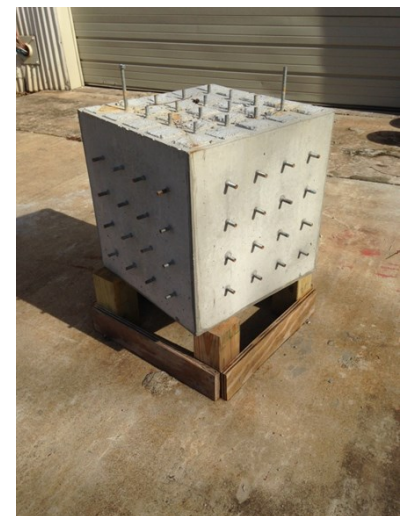
Sample triaxially-restrained ASR expansion cube
