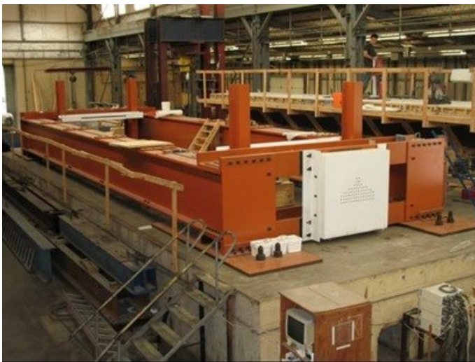
Prestressing bed at Ferguson Lab
