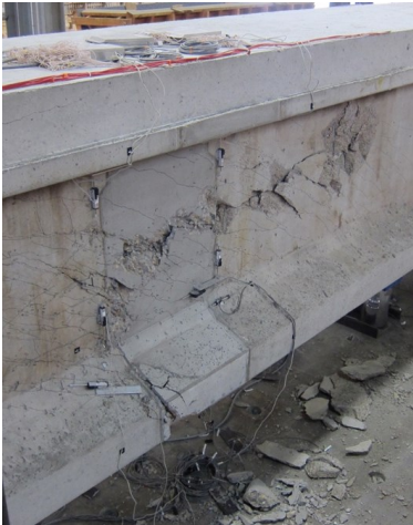
Spliced girder test specimen after failure
