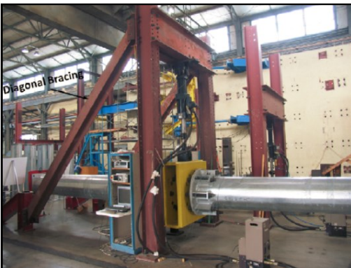
Portal loading frame used in previous fatigue studies in HMIPs at Ferguson Lab
