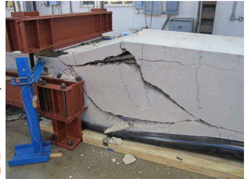
Uniform load testing using an air bag
