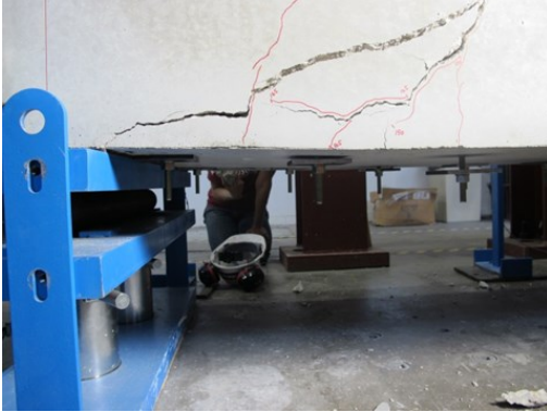
Expansion anchor shear retrofit
