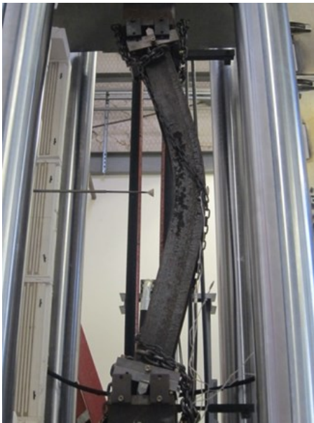
Buckled W4x13 column
