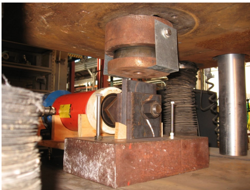
Slip test setup
