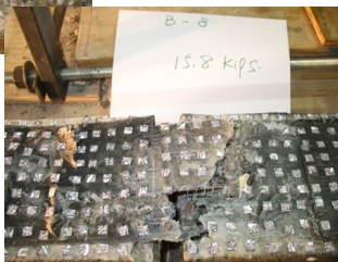
Right: FRP rupture failure mode
