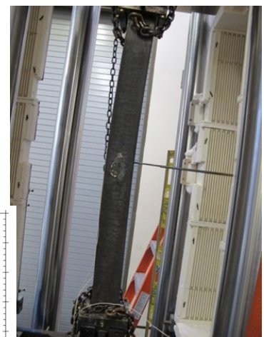
Buckled column at 700°C (above) and corresponding load-deflection plot (left)
