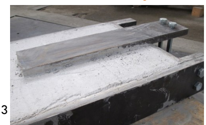
Composite specimen before (above) and after (below) concrete casting
