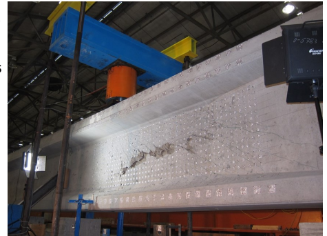
Failure of girder 5 showing vision system targets
