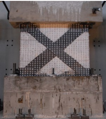
Retrofitted column (above) and masonry wall (below) after testing
