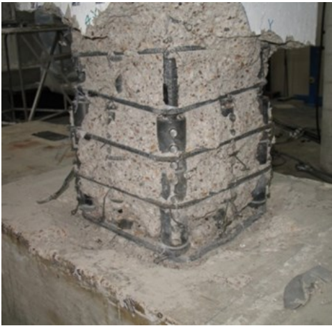
Retrofitted column (above) and masonry wall (below) after testing
