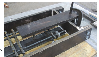
Composite specimen before (above) and after (below) concrete casting
