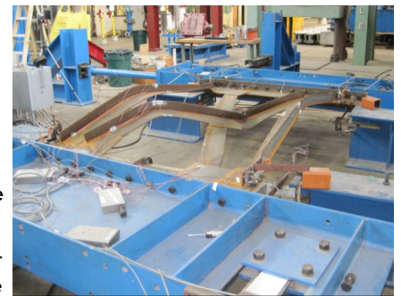
Cross frame stiffness test setup with unequal leg X frame
