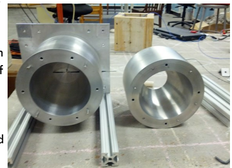
The cannon (ellipsoidal reflector) for nondestructive testing
