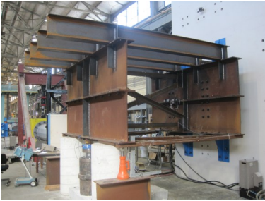
Cross frame fatigue setup with X frame
