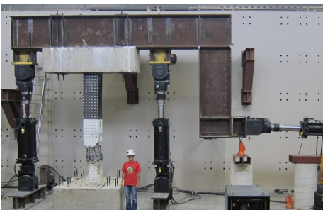
Repaired RC column after lateral cyclic and vertical load tests
