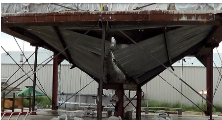
The floor slab at the moment of collapse
