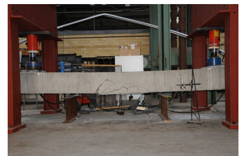
Info-only anchorage testing: Dramatic failure of a non-code compliant splice at a devastating 30 kips
