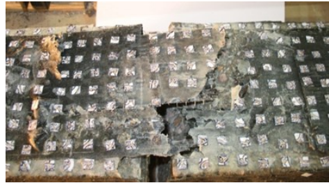
Below : Failure modes - FRP rupture (left) and anchor failure (right)
