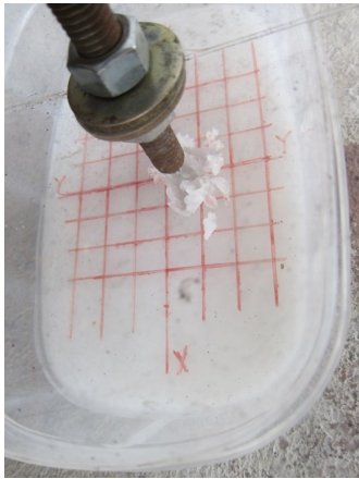
Wireless mechanical monitoring device (wax box) showing one week of recorded data
