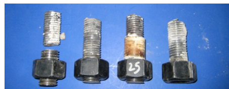
Failed connectors (adhesive anchor) from the first four tests
