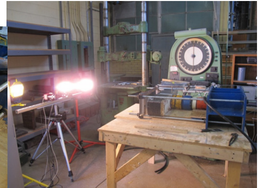
Setup for the test of the FRP-strengthened beam.
