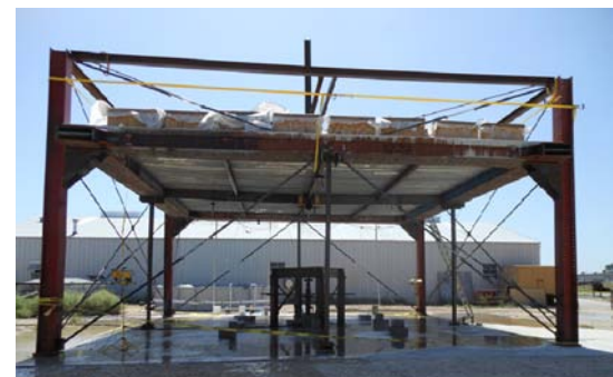
You can note there is a column missing from the middle of the structure. The structure did not seem to mind.
