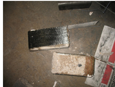
Below: Anchor failure (left) and FRP rupture failure (right)
