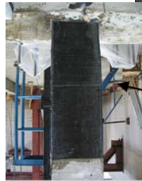
Partially-retrofitted masonry wall showing the concrete ring around the lower two courses of brick
