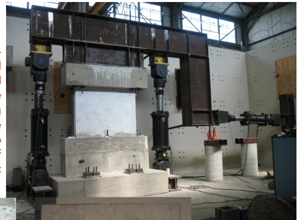
Partially-retrofitted masonry wall showing the concrete ring around the lower two courses of brick
