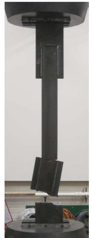
Right: Fatigue failure of a double angle cross frame - The fatigue tests were all that they were cracked up to be...
