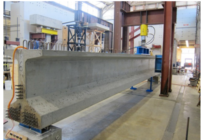
Testing at the service load of an 0-6374 beam
