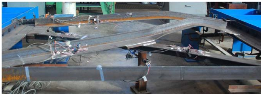
Below: Failure of an X-type cross frame
