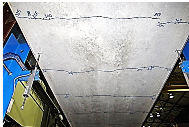
Testing at the service load of an 0-6374 beam
