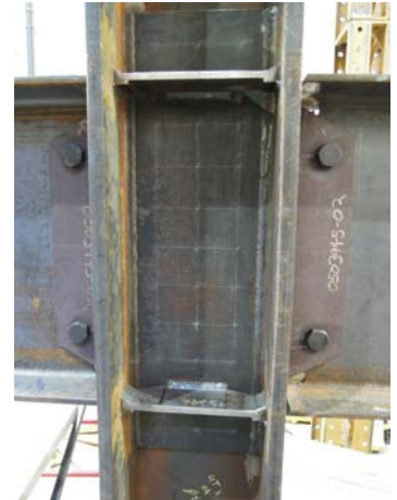
Column panel zone of WUF-W moment connection
