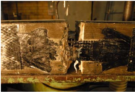
These beams are failing at a load of about 10 kips
