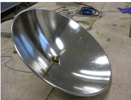
Parabolic dish and microphone for air-coupled sensing
