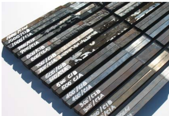
Coupons after cooling down with CIA, CIB, CIW
