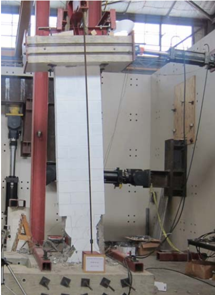
Above we can see one of the quasi-static masonry wall specimens tested at FSEL.
