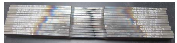
Tension coupons tested at high temperatures
