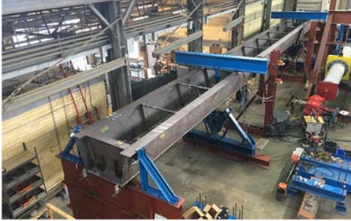
Tub Girder Test Setup
