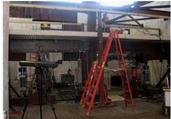
Test Setup at 9% Inter-story Drift
