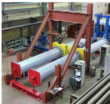
Figure 1: Test setup for fatigue tests.
