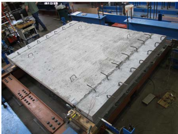
Failure of Closure Pour Strip due to Poor Confinement at Corners
