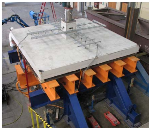
Uniformly Distributed Load Test Configuration
