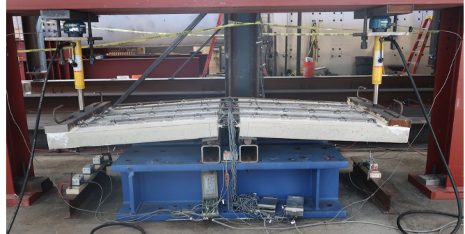
Test specimen after failure in four-point negative bending test
