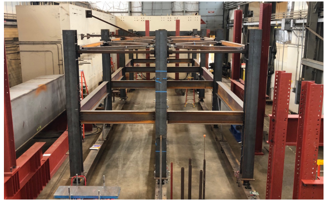
Two-by-three bays of steel gravity framing
