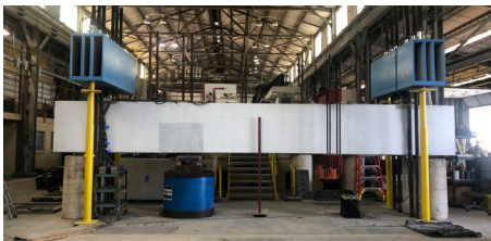
Deep beam testing setup
