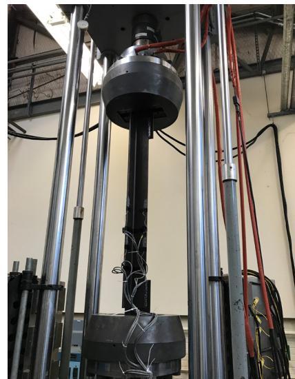
Eccentrically connected single-angle specimen examined as part of the original NCHRP study.
