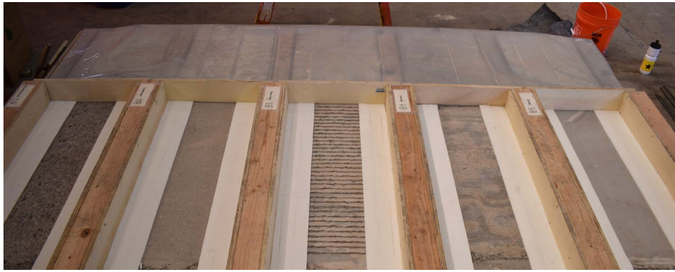
Beam specimens with various interface conditions
