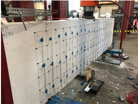
Beam during test with motion capture system
