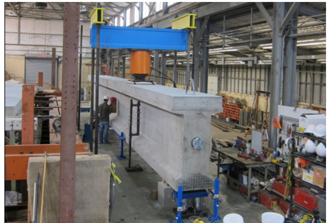
Post-tensioned concrete girder at FSEL
