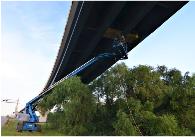
Research team instrumenting a horizontally-curved bridge with strain gages and wireless monitoring equipment
